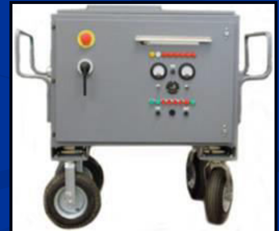
Robins Air Force Base DC Power Supply 28.5V, 600A, Triple Input Aircraft Engine Starting
