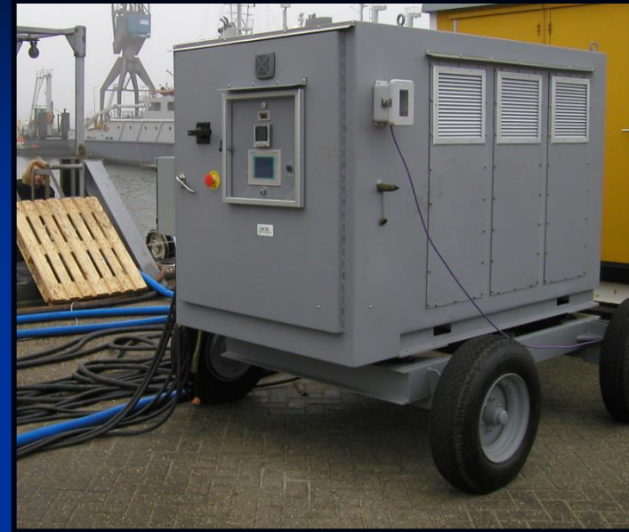
Dutch Navy Battery Charger and Discharger for Submarine Batteries 260KW and 520KW
